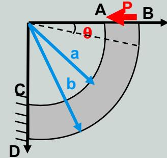
$$u(\theta = 0) = L = \frac{D \pi}{E} \quad D = -\frac{P(a^2 + b^2)}{a^2 - b^2 + (a^2 + b^2) \log \frac{b}{a}}$$
